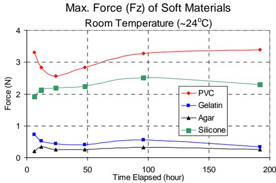
Figure 6: Change in insertion forces, i.e. resistances over time (at 6hr, 12hr, 24hr, 48hr, 96hr, & 192hr intervals) when the phantoms (PVC, gelatin, agar, & silicon rubber) are kept on the shelf at room temperature at about 24°C.
