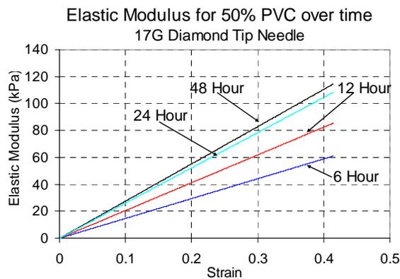
Figure 8: Change in Young’s modulus of 50% PVC material at different time intervals (6hr, 12hr, 24hr, & 48hr).
