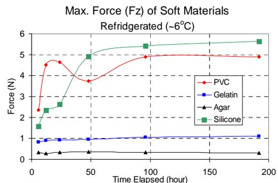
Figure 5: Change in insertion forces, i.e. resistances over time (at 6hr, 12hr, 24hr, 48hr, 96hr, & 192hr intervals) when the phantoms (PVC, gelatin, agar, & silicon rubber) are kept refrigerated at 6°C temperature.
