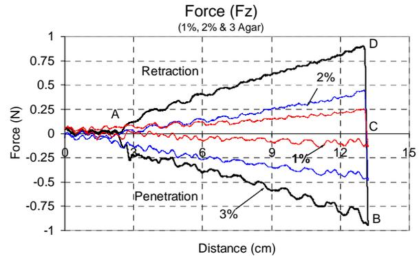
Figure 4: Forces in z-direction while inserting needle in agar phantom with 1%, 2%, and 3% concentrations.
