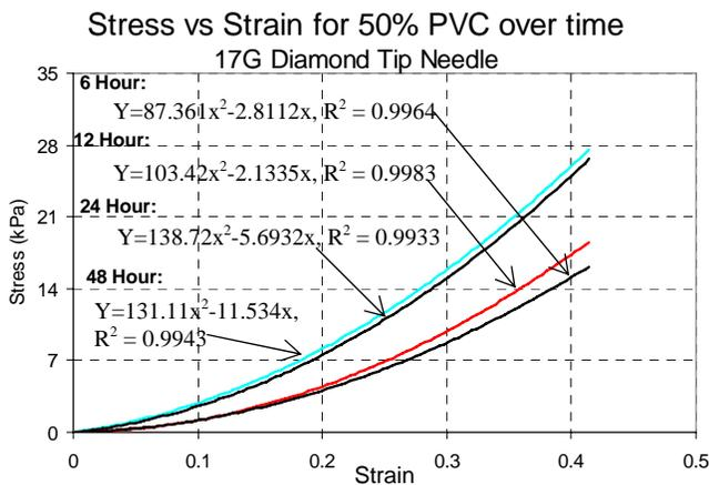
Figure 7: stress vs. strain plots of 50% PVC material at different time intervals (6hr, 12hr, 24hr, & 48hr).
