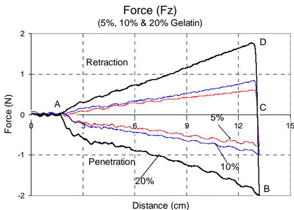
Figure 3: Forces in z-direction while inserting needle in gelatin phantom with 5%, 10%, and 20% concentrations.
