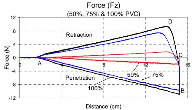
Figure 2: Forces in z-direction while inserting needle in polyvinylchloride (PVC) with different percentages of plasticizer (50%, 75%, and 100%).
