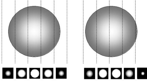
**Figure 1.** Models illustrating the variations in appearance of a sphere on simulated CT image slices caused by changes in position of the central image slice. Left pair: central image slice intersecting exact center of sphere. Right pair: central image slice shifted one-third of the slice thickness from the exact center of sphere.
